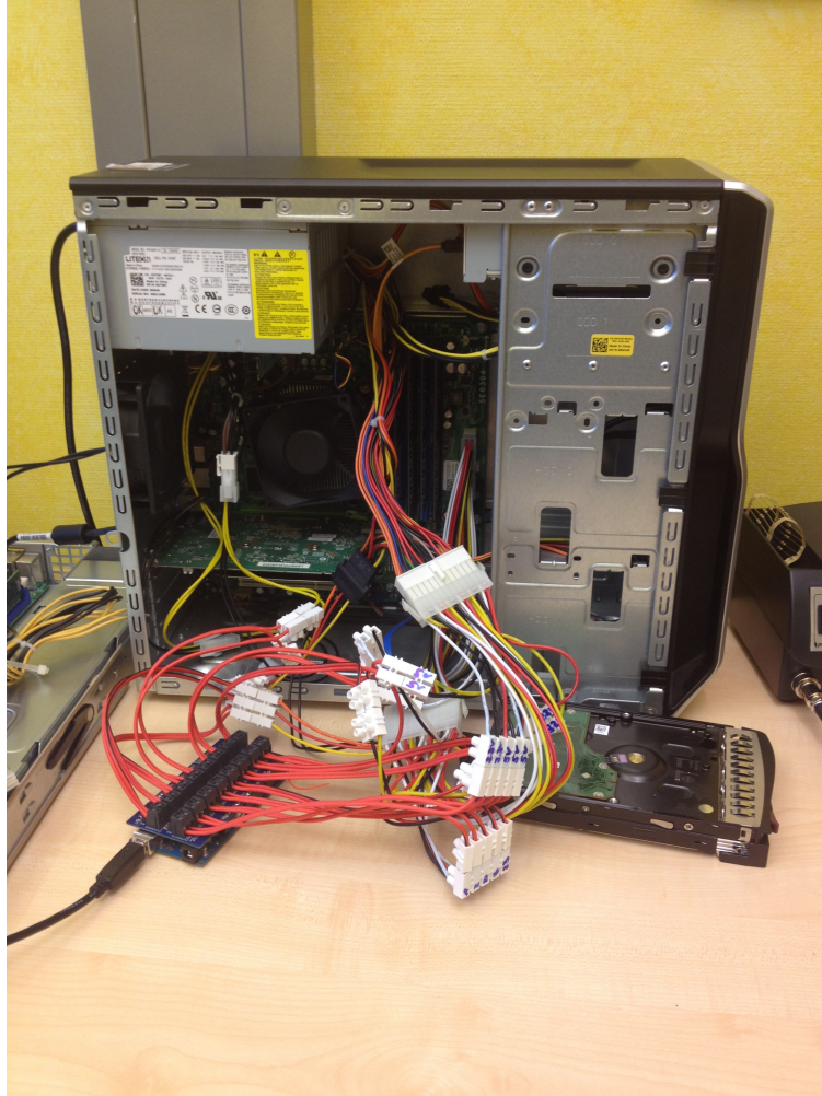
Figure A.7.1: The measurement device installed into a desktop machine.
