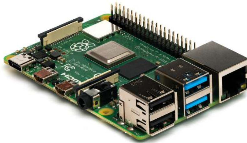
Figure 3.1: The Raspberry Pi 4 [H.a]
