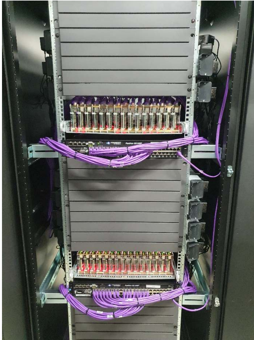
Figure 6.2: Both layers of installed Raspberry Pis and rack panels
