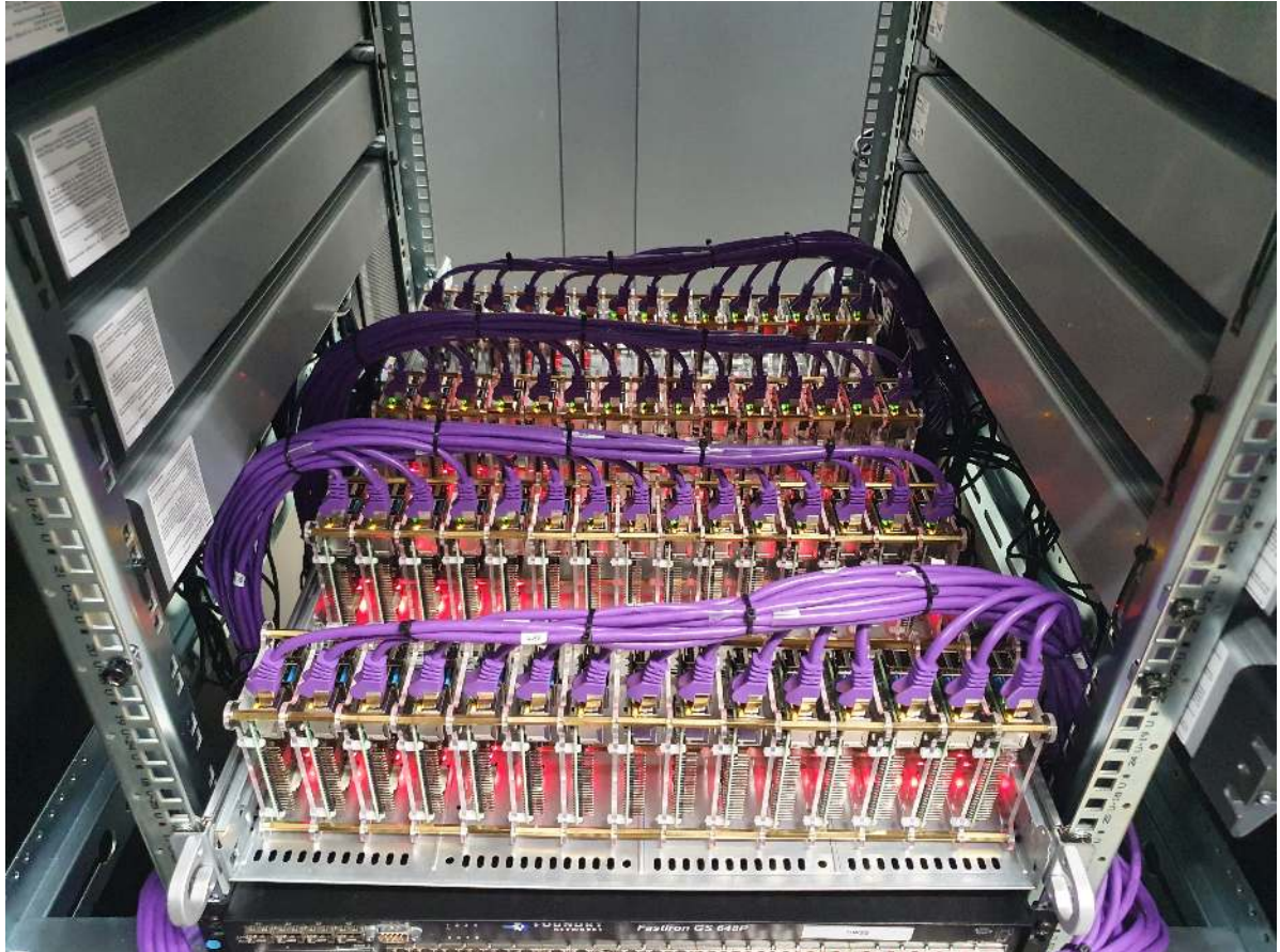
Figure 6.1: One layer of installed Raspberry Pis
