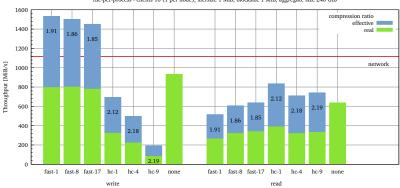
file-per-process - clients 10 (1 per node), xfersize 1 MiB, blocksize 1 MiB, aggregate size 240 GiB
