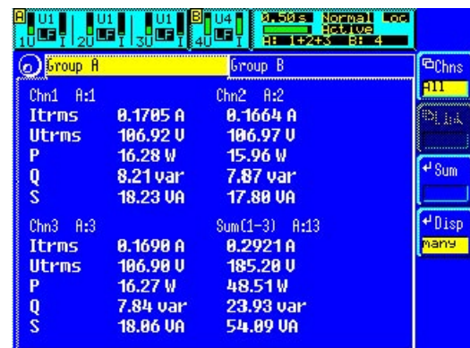
Fig. 5.1: Display screenshot of the ZES ZIMMER LMG450 [33]
